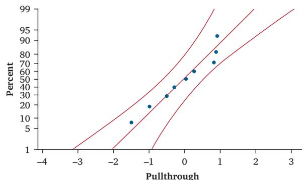
**Figure 1.** Individual distribution identification analysis assessing variance between mean peak deformation force values for the pullthrough wires.
