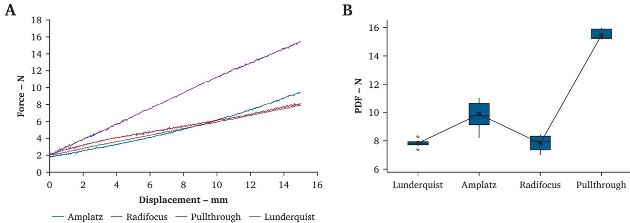
**Figure 2.** (A) Composite graph indicating typical deformation trends for each wire configuration, emphasising the linear graph slope and high peak deformation force (PDFs) needed for the Pullthrough wire during deformation. (B) Box plot indicating the range of PDFs across the four wire configurations.
